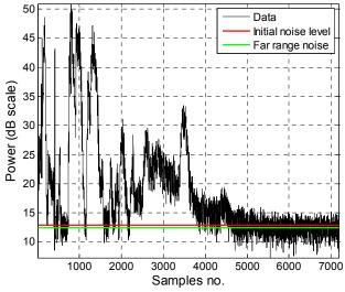
**FIG. 1** Received power as a function of range at the elevation angle of 0.5 deg. The number of samples at each range position is 15 and the range sample spacing is 60 m. The initial and "true" noise values are indicated with a red and green line, respectively. This data was collected using the NWRT PAR in Norman, OK.
